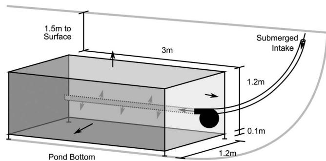
**Fig. 1.** Submerged denitrifying bioreactors for treatment of nitrate in wet detention ponds. Arrows indicate flow paths from intake, through the pump, and radially from the perforated pipe, through the woodchips, and out of the bioreactor. The metal frame was lined with geotextile fabric and secured with cable ties to contain the woodchips.
